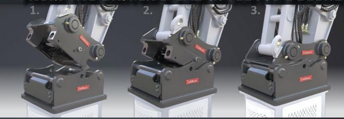
OilQuick is an automatic quick coupler system which allows hydraulic work tools to be connected and disconnected from the driver's cab. The operator can change between various work tools within seconds.
